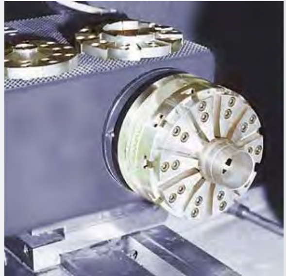
Circular grinding with permanent circular magnetic chuck. In this application upto 300 different workpieces can be machined using 4 sets of pole raisers.
