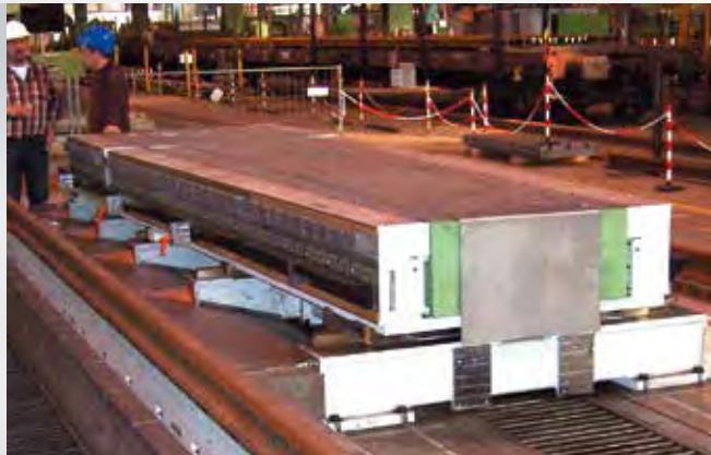
B ) Welding preparation of heart sections to length 2 x 5 m
