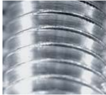
Smooth surface due to excellent lubrication
