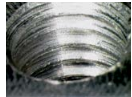
Tap with TiCN layer in AISi7
