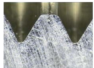
Thread profile made with a special former
