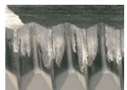
Example of weld formations
